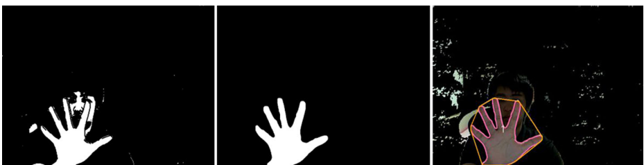
Fig. 27 (left) Skin extraction after Canny Edges segmentation (center) Contour extraction, keeping only the largest contour, effectively removing face region (right) Hull extraction without face
