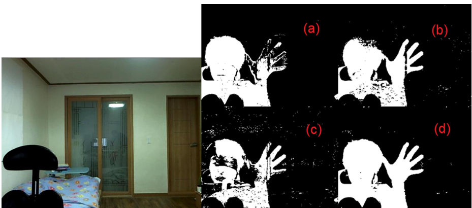
Fig. 19 ( left ) Static background image ( right ) After background subtraction with current image a Y channel b Cr channel c Cb channel d Combine 3 channels by addition operation
