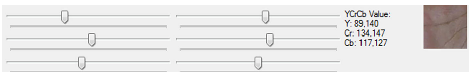
Fig. 31 One click calibration method and scroll bar to fine tune threshold value
