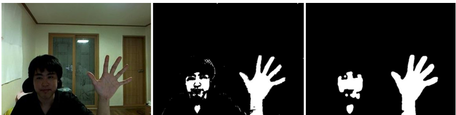
Fig. 21 (left) Original frame (center) Skin color extraction using narrow threshold (right) Morphology operation and Gaussian smoothing
