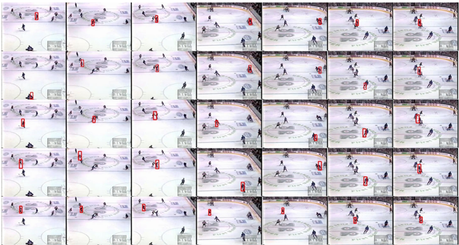
Fig. 4 Tracking results over the Hockey1 sequence. From top to bottom: 2MCMC-PF, ASAMC, WLMC, HMC, and AMCMC, the sample frames are #69, #303, #320, #458, #470, #510, #512 (from left to right)
