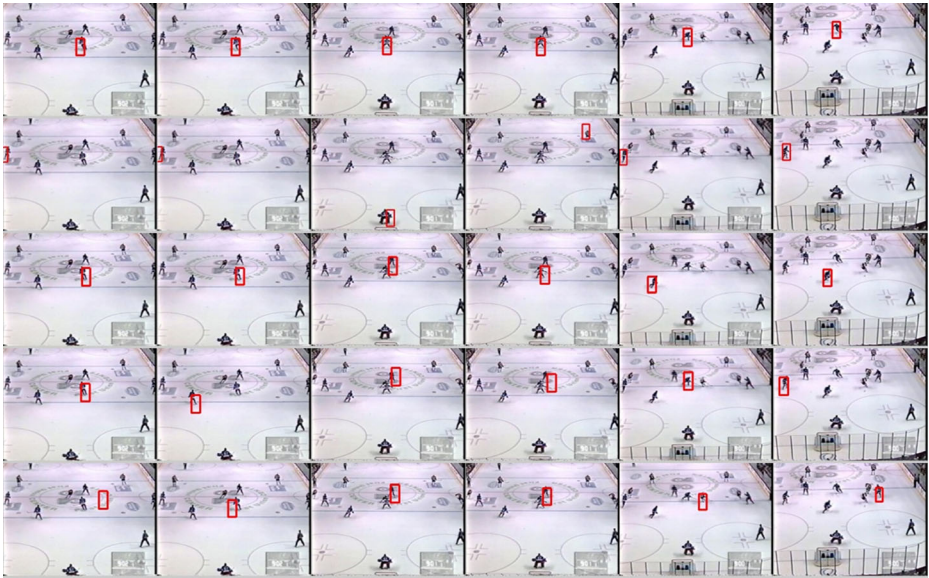
Fig. 6 Tracking results over the Hockey2 sequence. From top to bottom: 2MCMC-PF, ASAMC, WLMC, HMC, and AMCMC, the sample frames are #23, #24, #39, #40, #61, #82 (from left to right)
