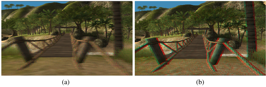
Fig. 11 a Final interlaced image for the auto-stereoscopic display and b the same scene with an anaglyph system for any conventional display
