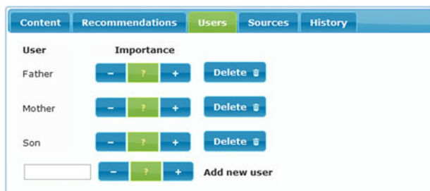
Fig. 6 The Users tab of the user interface. Every user in the OMUS system is associated with an importance factor that can be changed according to the desired context
