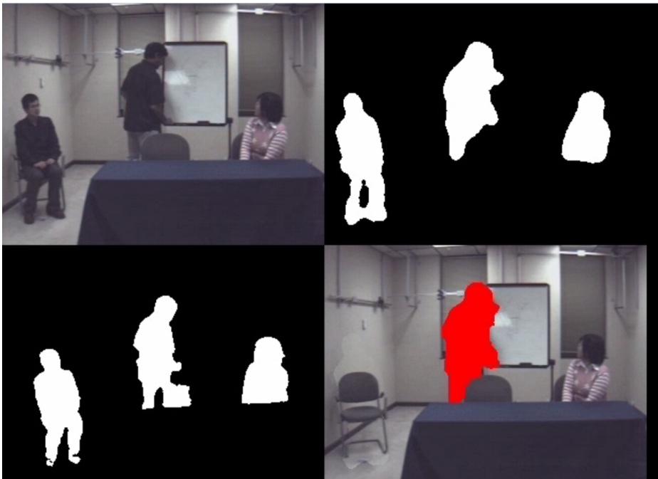
Fig. 14 Using thermal and visible light camera fusion algorithm to improve human segmentation with applications in privacy protection. The top left image is from the original video, the bottom left image is the background subtraction from thermal camera, and the top right is the segmentation result from visible-light camera. The bottom right image is the final result by removing the person on the left and obfuscating the person in the middle, both benefited from an accurate fused segmentation result
