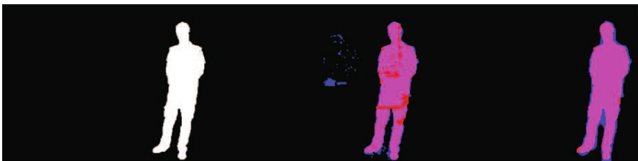
Fig. 13 Quantitative measurement of the segmentation result. Left : ground truth; middle : color segmentation; right : fused segmentation
