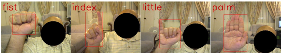
Fig. 5 Face detection and subtraction as well as hand posture detection (in red square)
