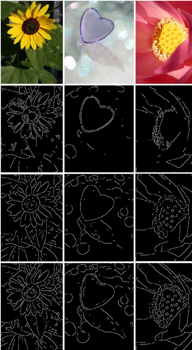
Fig. 2 Comparison for edge detection using canny detector. From top to bottom: Original images, RGB color edges, color boosted edges based on [36] and color boosted edges based on our method
