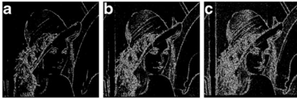
Fig. 5 Difference images with embedding rate of a) 0.2 bpp, b) 0.3 bpp, c) 0.4 bpp
