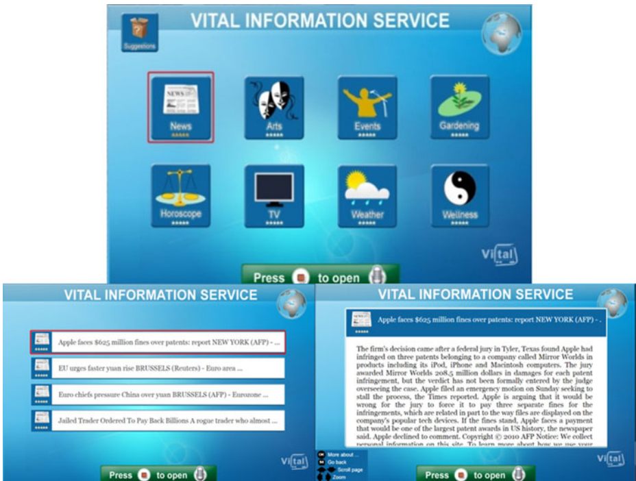
Fig. 8 On the top, a screenshot of the start page of the Information Service is displayed. Preselected topic areas are distinguished by big icons and ordered by users' preference that may change after usage. Below, two screenshots of the navigation through the content are shown
