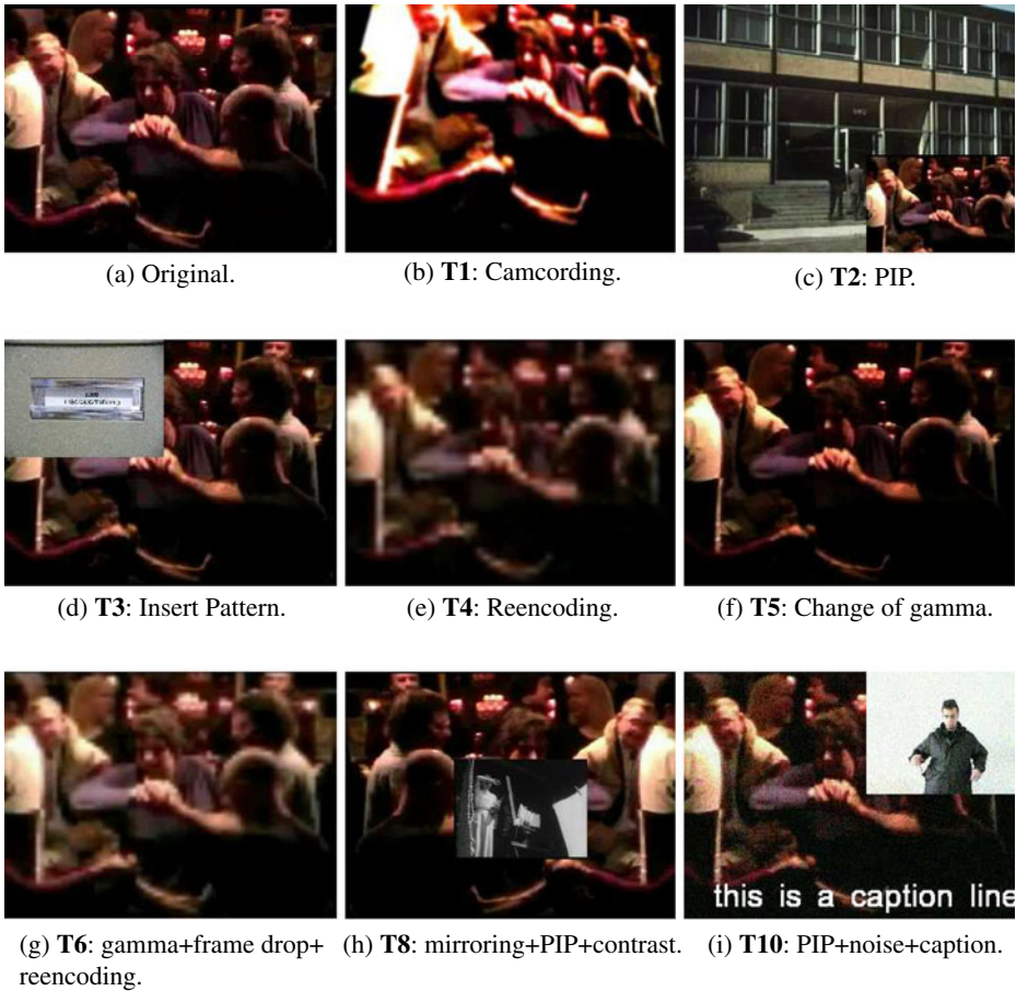
Fig. 14 Example of transformations in TRECVID 2010. a Frame from a reference video, b–i same frame from each query video for the eight visual transformations
