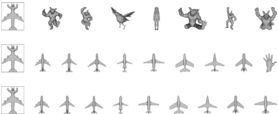
Fig. 11 Another partial matching example showing the top-7 retrieval results using RPU ( 1st row ) method and the top-9 retrieval results using ZFDR ( 2nd row ) and CBR-ZFDR ( 3rd row ) methods. The first model in each row is the query model
