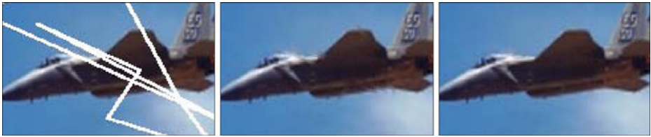
Fig. 3 Comparison between the isotropic and anisotropic models. From left to right: damaged image, inpainting result obtained using the isotropic model with PSNR=44.1 dB, where blurring at edges are visible, and result obtained using the present method with PSNR=50.2 dB and improved visual quality
