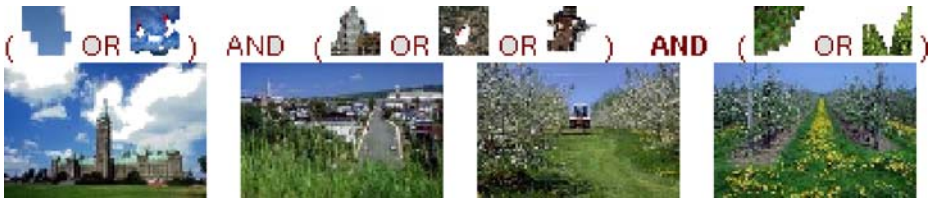
Fig. 5 First row: a query consisting of a Boolean composition of regions. Second row: matching images. (Courtesy of J Fauqueur)
