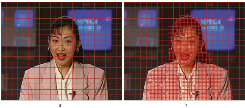
Fig. 2 A comparison of FSBM and VSBM a block distribution of FSBM algorithm; b block distribution of VSBM algorithm
