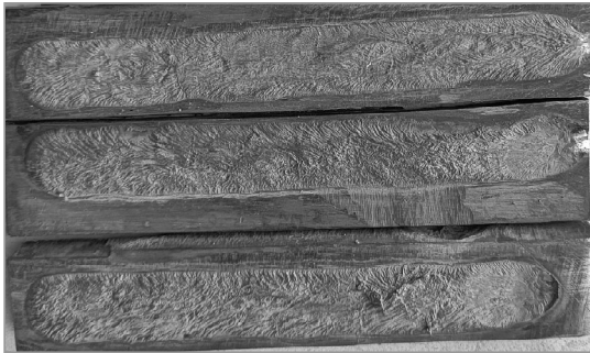
Fig. 2. Appearance of titanium nickelide beads surfaced on titanium.
