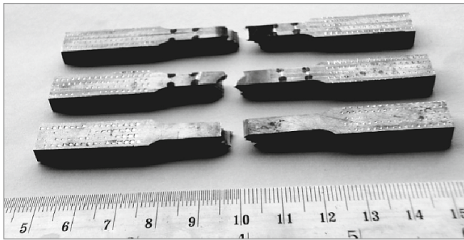
Fig. 5. Appearance of fractured specimens after tensile tests.
