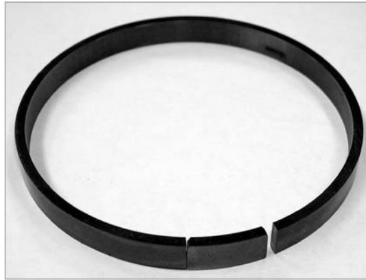
Fig. 1. A ring cut out from a sleeve and a sample for analysis cut across the ring generatrix.
