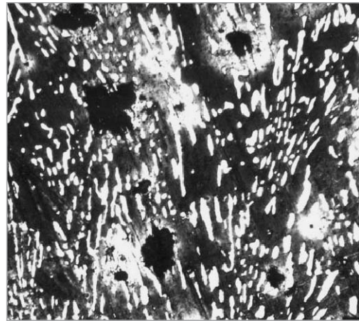
Fig. 6. Composite structure of mottle with 4.5 wt.% Cu. \times 200 .
