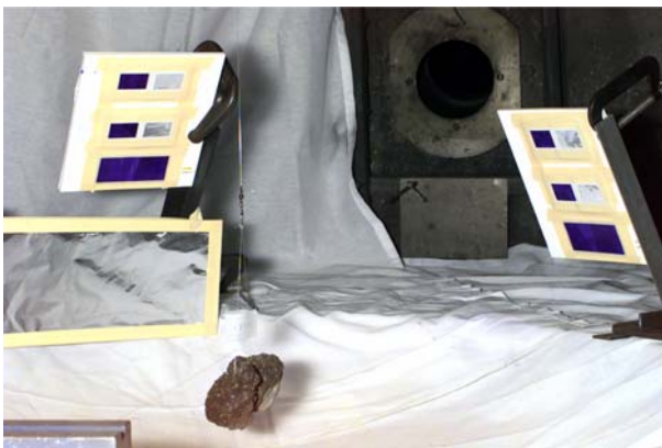
Figure 1. Anhydrous basalt target suspended in the AVGR chamber with two of the passive detectors, each containing two 7 \mu\text{m} , two 13 \mu\text{m} , and one 51 \mu\text{m} foils, deployed upstream from the impact. The projectile enters the AVGR chamber through the circular port in the top right of the image. In this case, a larger piece off Al-foil was deployed below the foil detector, to monitor the distribution of punctures over a larger area.
