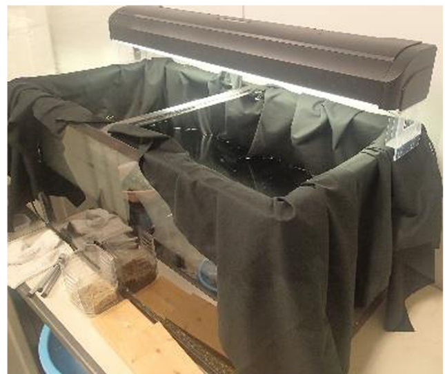
Fig. 3 Experimental setup (OLYMPUS uTough 8000 underwater camera, INON LE700-W/S LED lights, and SLIK SBH-320DS PTZ)
