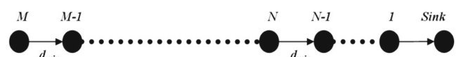
Fig. 2 The queuing model of relay with minimal transmission range of d_{min} and maximum transmission range Nd_{min}
