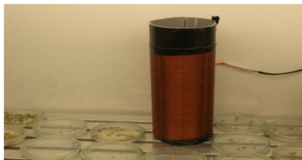
Fig. 1 A magnetic coil that had been used in study of magnetic field effects on callus induction derived from embryo culture in bread wheat ( Triticum aestivum . L) genotypes. The petridishes should be placed into the device
