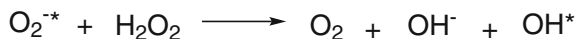
Fig. 1 Fenton reaction by which \text{H}_2\text{O}_2 forms hydroxyl radical in iron rich environment
