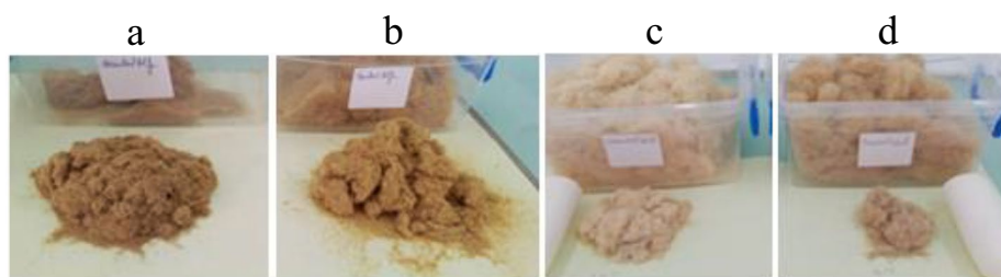
Fig. 2. Untreated and treated samples fibers: untreated (a) and treated (b) Alfa; (c) untreated (c) and treated (d) Sisal.
