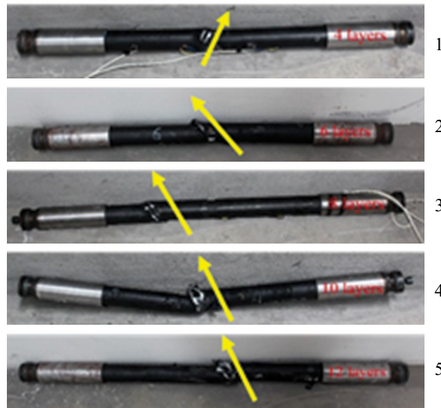
Fig. 4. Fracture morphologies of TCPs with 4 (1), 6 (2), 8 (3), 10 (4), and 12 (5) reinforced inner layers.
