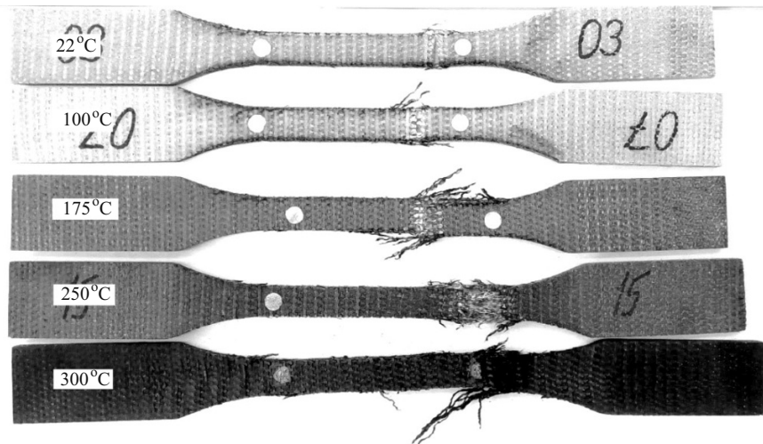
Fig. 5. View of rupture and magnitude of irreversible deformation of glass-fiber plastic samples at different temperatures.
