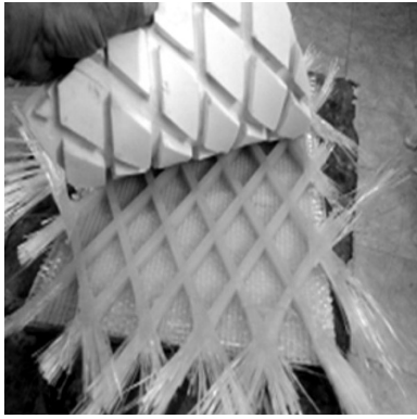
Fig. 4. Separating the silicon mold from the core.
