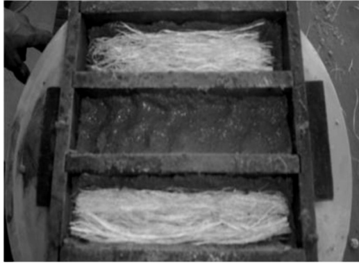
Fig. 2. Mold for specimen preparation — top view.
