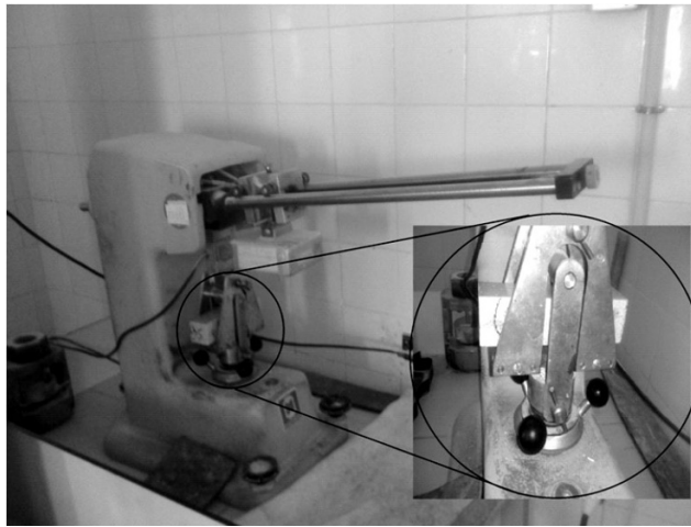
Fig. 3. Three-point bending test machine.
