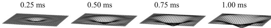
Fig. 9. Deformed shape of the 400-mm laminate after a 7.2-m/s impact in the absence of preload.
