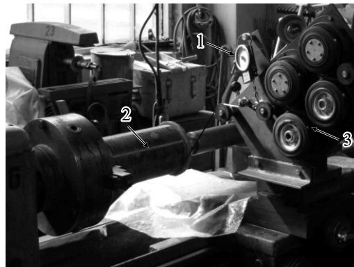
Fig. 1. Winding equipment: 1 — dynamometer; 2 — specimen; 3 — pretension device.
