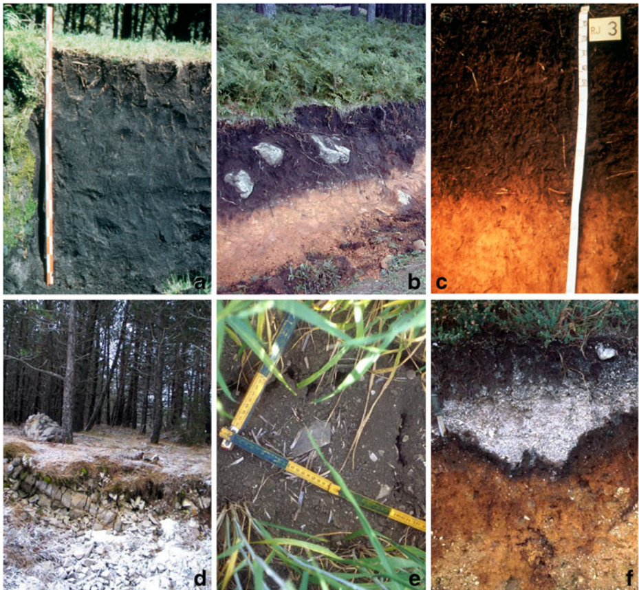
Fig. 5 Some natural soils with stable C forms and potentially useful as models for the elaboration of Technosols derived from waste. a ali-humic Umbrisol (Galicia, NW Spain); b alu-Andic Andosol (Galicia; NW Spain); c umbric Ferralsol (Minas Gerais, Brasil); d rendzic Phaeozem, (Eslovenia), e grumic Vertisol (Sevilla, Spain); f albic Podzol (Galicia, Spain)
