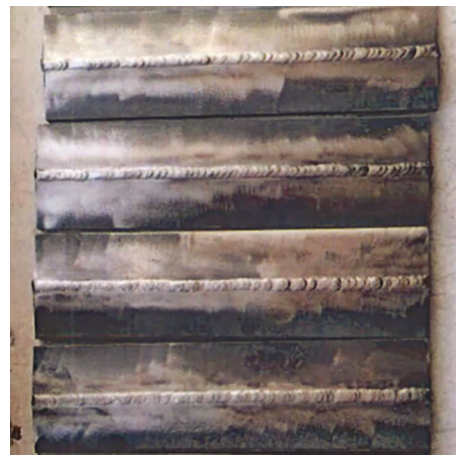
Fig. 3 Appearance of welded joints manufactured from 10-mm-thick sheets of the nickel alloy grade CrNi 62 MoCh 2 -VI (EC 199-VI) at the Research Institute of Chemical Engineering
