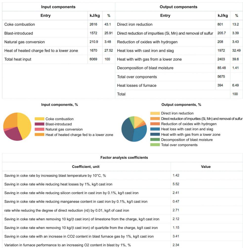
Fig. 4 Fragment of a web page visualizing the calculation of heat balance in the BF lower part
