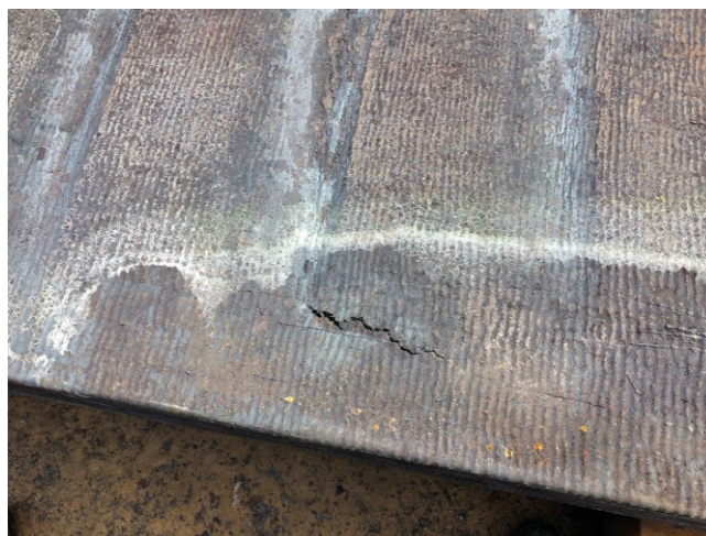
Fig. 2 Defect: “cracks along the scab”
