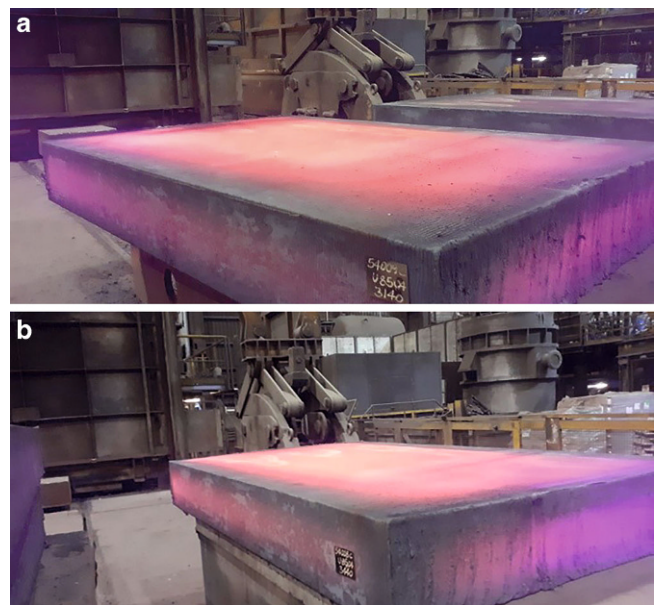
Fig. 10 Surface of 400-mm-thick slabs cast after introducing the technology
