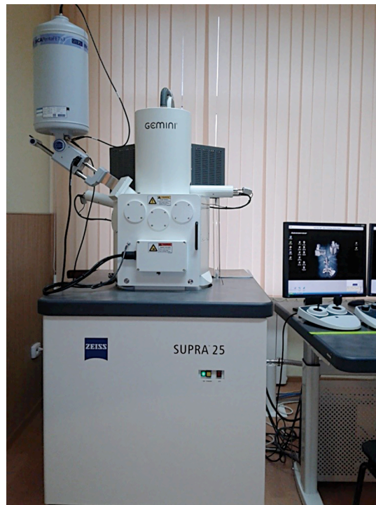
Fig. 2. ZEISS SUPRA 25 scanning electron microscope.
