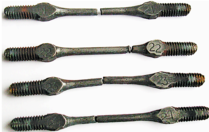
Fig. 3. Specimen after high-temperature breakage.
