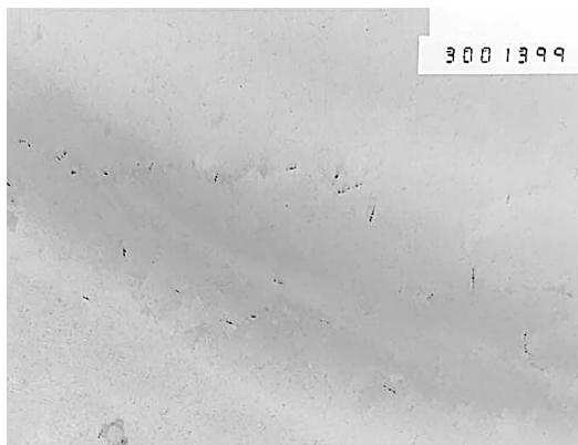
Fig. 4. Typical form of second type of carbide precipitates on hot-rolled steel melt No. 1 (light-field image, \times 30,000 ).
