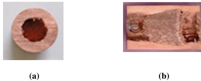
Fig. 2. Fracturing in the transverse (a) and longitudinal (b) cross-sections of the rods obtained by radial-shear rolling.
