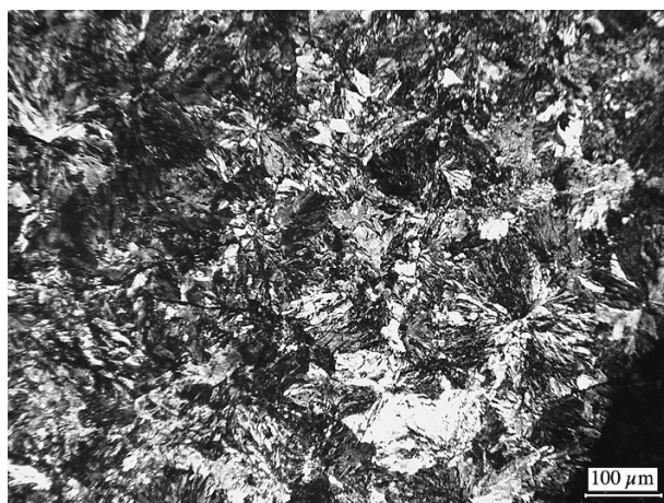
Fig. 1. Microstructure of CBC steel 35KhGSA metal surface.
