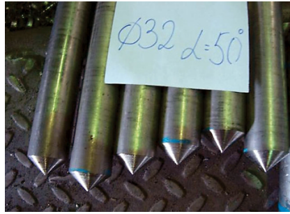
Fig. 1. Billets with a diameter of 32 mm and a half end cone angle of 50°.
