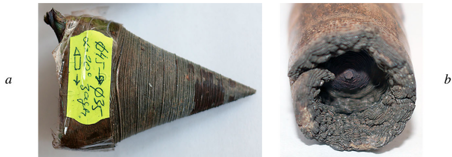
Fig. 7. Ends of workpieces with cone angles of 40^\circ (a) and 100^\circ (b) after rolling.
