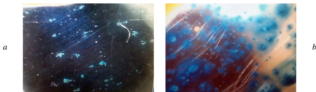
Fig. 3. External surface appearance of rolled product specimens No. 1 (a) and No. 2 (b) with E = -36 mV; picture through layer of electrolyte.
