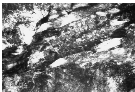
Fig. 1. Microstructure of steel 30Kh2AF in hot-rolled condition.
