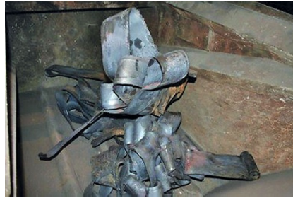
Fig. 1. Band of metal extricated from the drum of the piercing-mill roll.
