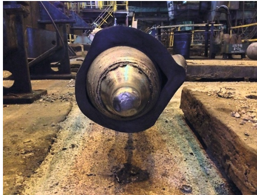
Fig. 2. Lap formation on the back end of the hollow.
