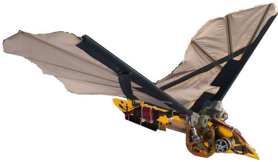
Fig. 2 Constructed FMAV and its main parts
