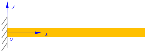
Fig. 3 Equivalent beam model of the space truss
