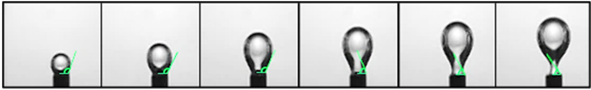
Fig. 18 Bubble formation process with the contact angle for the circular needle with 1200 mlph flow rate and 5 cm liquid height above the needle
