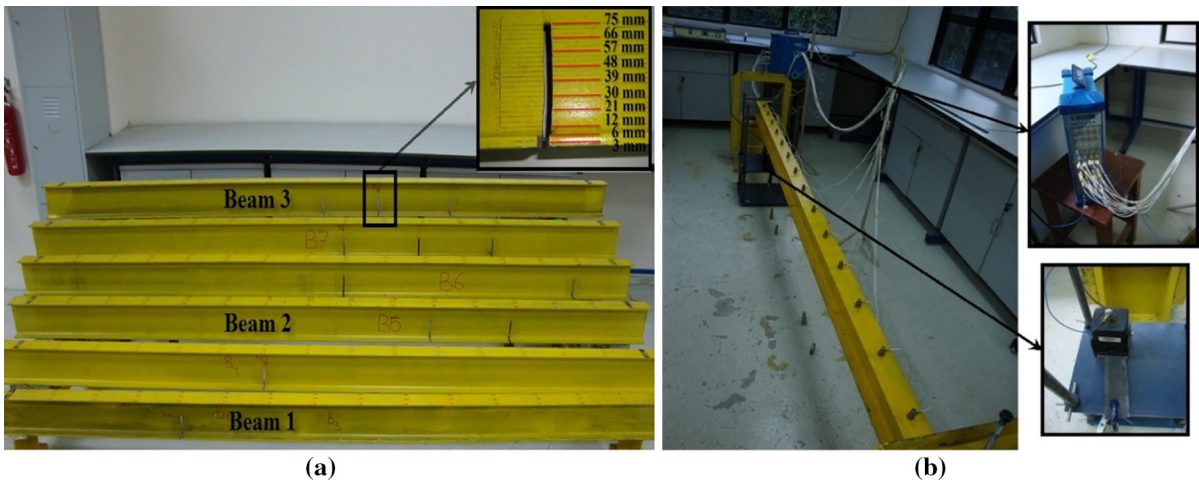
Fig. 10 Dynamic test in laboratory. a Damage locations of tested beams, b data acquisition system
