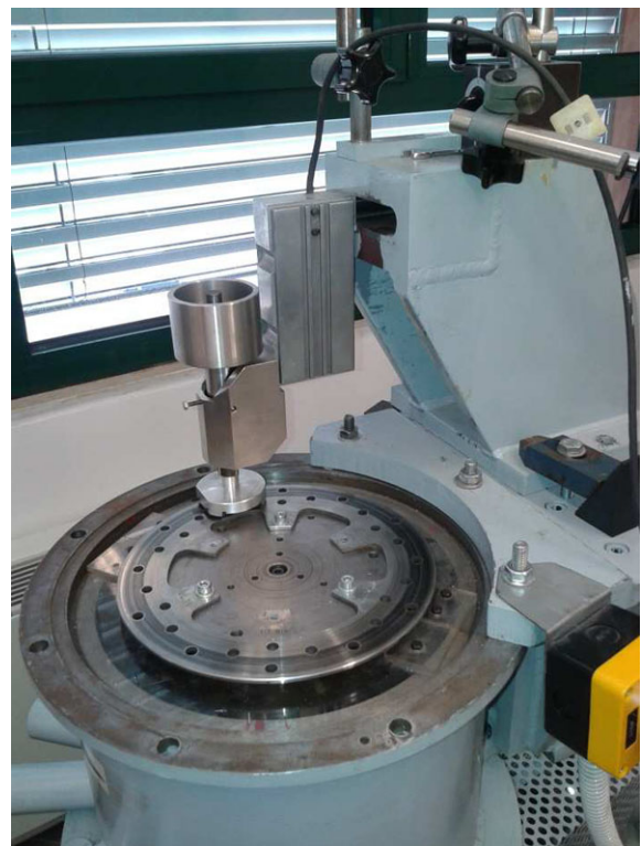
Fig. 8 Pad and disc fixed on the tribometer for friction tests
