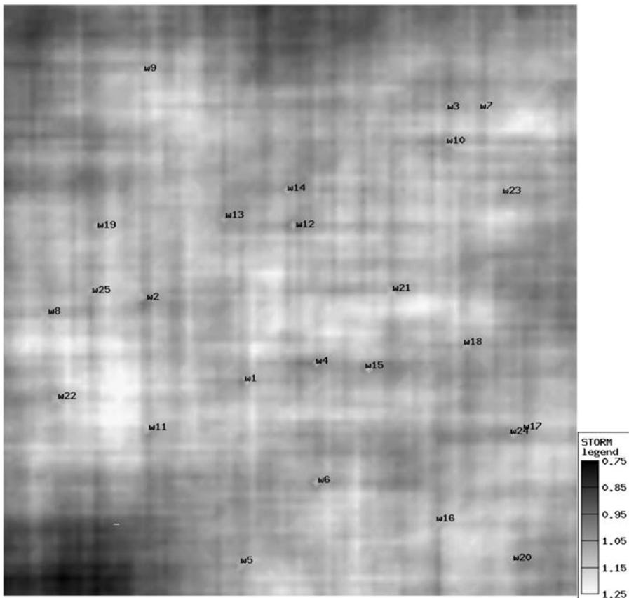
**Fig. 7** Ratio of the mean net/gross in conditional realisations to that of unconditional ones for the general model
