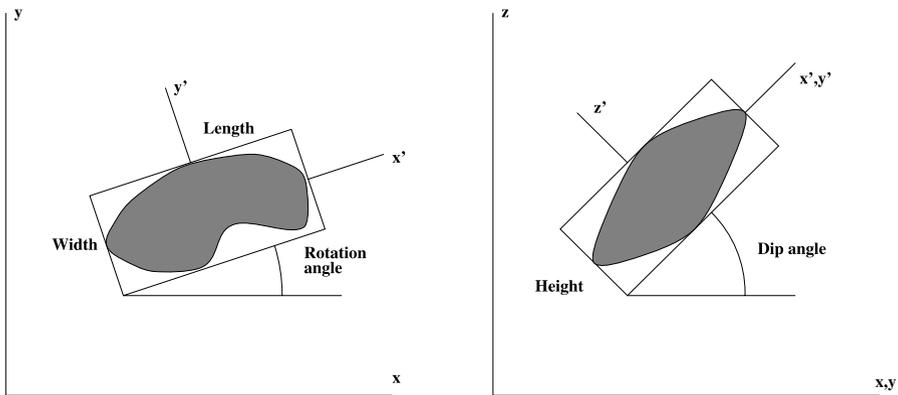
**Fig. 3** Basic geometry of the general model shown in the  $xy$ -plane (on the *left*) and a plane parallel with the  $z$ -axis (on the *right*)
