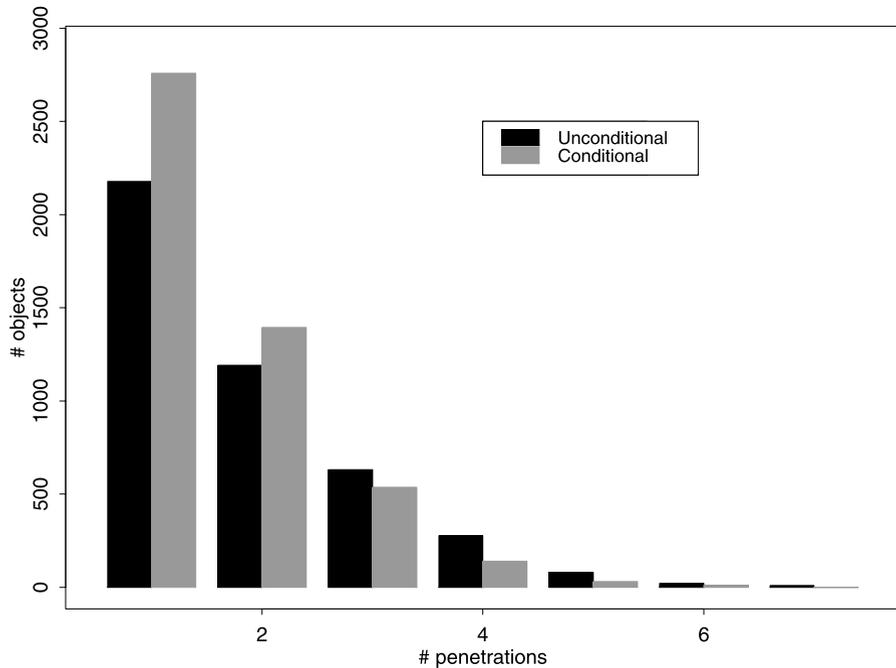
**Fig. 5** Number of well penetrations per object in conditional and unconditional realisations for the fluvial model
