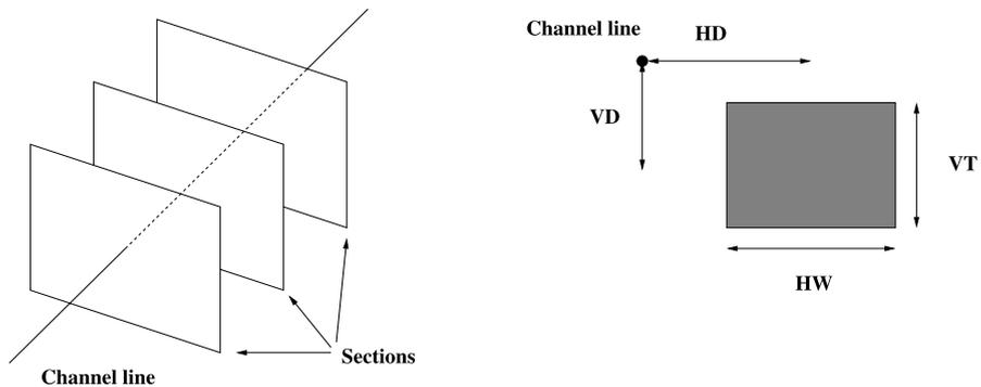
**Fig. 1** Basic geometry of the fluvial model showing the channel line and sections (on the *left*) and a section view (on the *right*)
