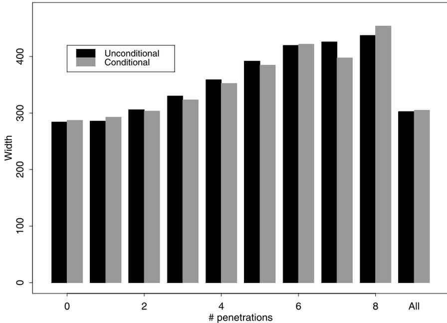
**Fig. 9** Width of objects against the number of penetrations in conditional and unconditional realisations for the general model. The *rightmost column* is the average width over all objects
