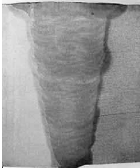
Fig. 4. Macrorecording of welded joint.
