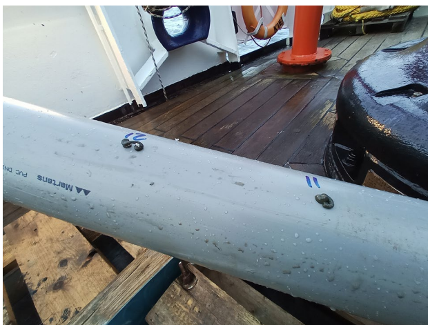
Fig. 4 Discharge of muddy material through boreholes in the core liner at location VH002 may be attributed to degassing upon pressure release (Photo taken by R. Usbeck)
